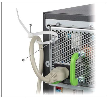
Figure 11: Using cable ties
